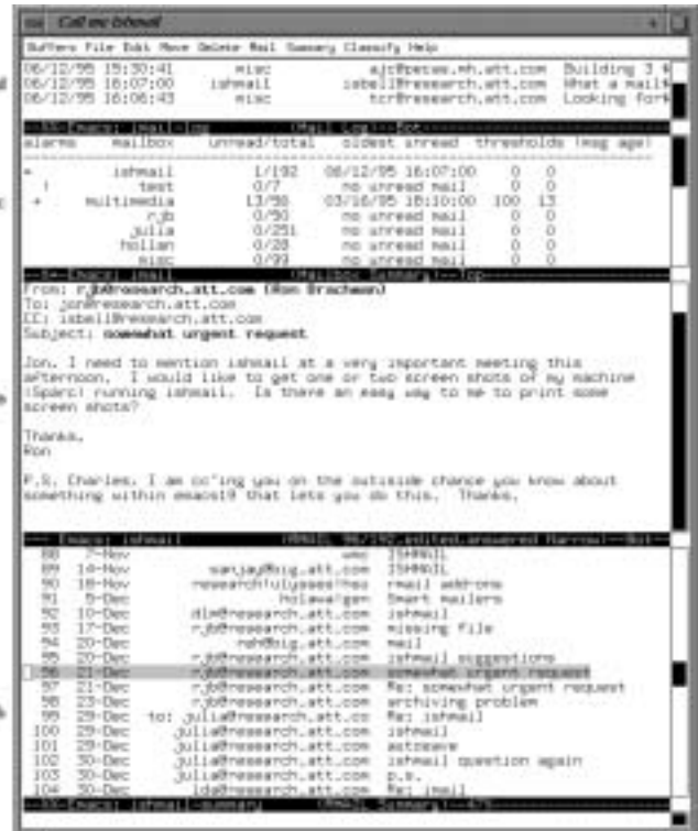
Figure 1: Ishmail User Interface. Four views: a) the current message, b) headers of the current mailbox, c) summary of mailboxes, d) log. Here, the summary view indicates why three mailboxes require attention and the log view indicates recent activity.
